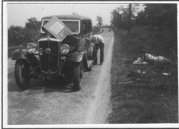
44. Puncture! Mr Moulton of Brickwall Farm Cottages is changing the tyre while my mother reads blithely nearby. The bonnet is open because this type of car had a toolbox inside the engine compartment on the near side.
