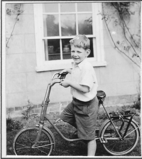
35. My brother, Adrian, with his Fairy Cycle, a very popular child's bicycle of the 1930s. It had solid rubber tyres and a single front brake in the form of a metal shoe which pressed down on the tyre.
